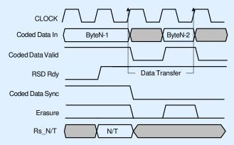
Note that the decoder will always take rsd\_rdy low for (at least) one cycle at the end of each codeword. However, if the rest of the decoder is ready this will not cause an overflow.
